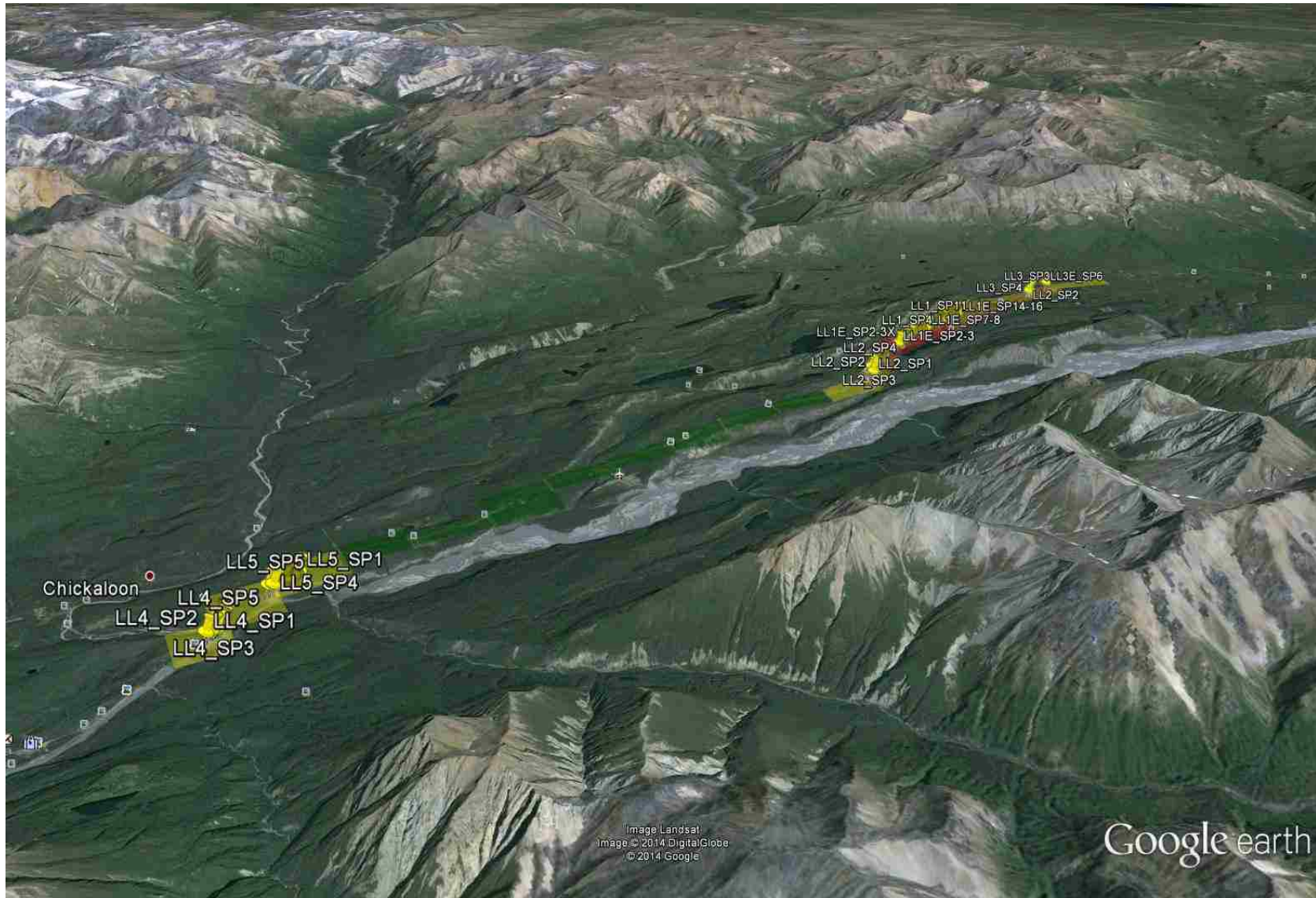
Figure 5.6: Glenn Highway survey site. The different shaded colors were for the priority of the sites, the yellow pins were scan positions. The priority colors were: Red->Green = Highest -> Lowest Priority
