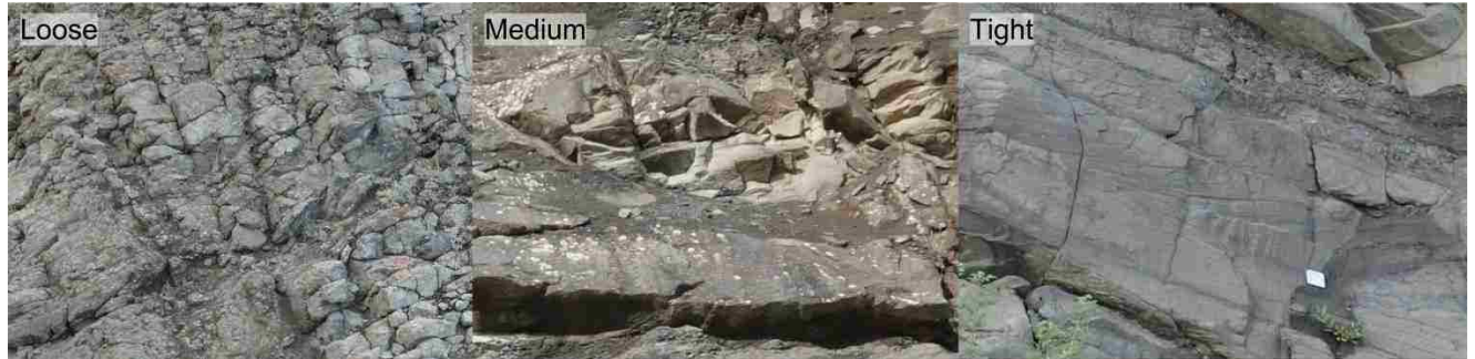
Figure 4.6: Generalization of the fracture aperture. Examples of each level, loose, medium and tight can be seen in Figure 4.7. (Nicholson, 2004)
